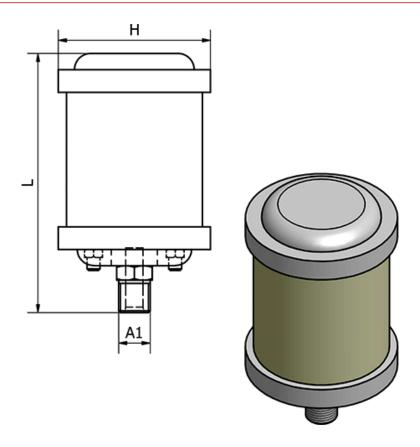
Flow I/min at 5 bar = 14000 H = 68.5 L = 184 Thread A1 = G 3/4"
